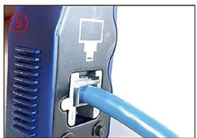
9.Put the plug into the tooland confirm push to the buttom.
