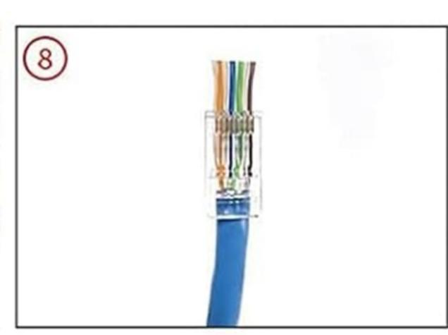
8. Pass the wires thru the connector and Perform sequence verification again
