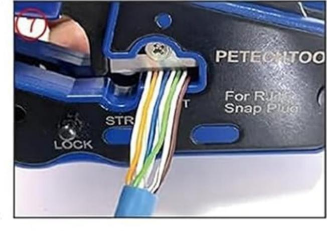
7. Trim the network cable neatly to make it easier to perforate.
