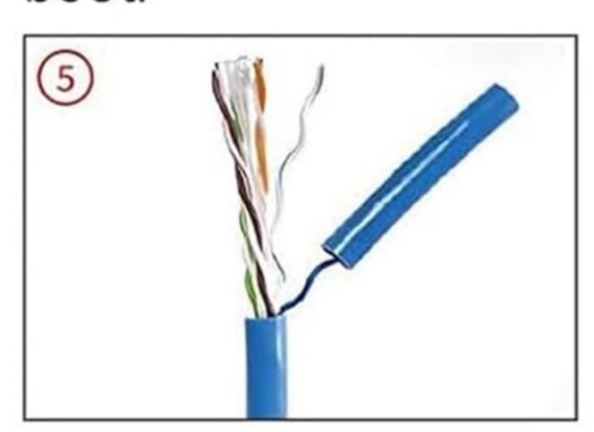
5. Separate the twisted pair and straighten it.
