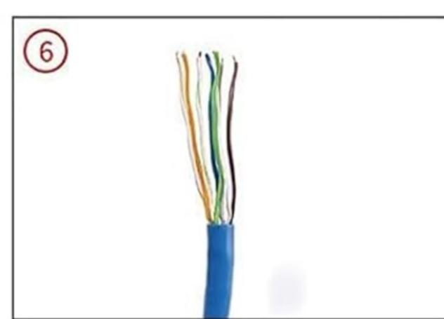
6.Arrange the wires according to the rj45 color "T568B"
