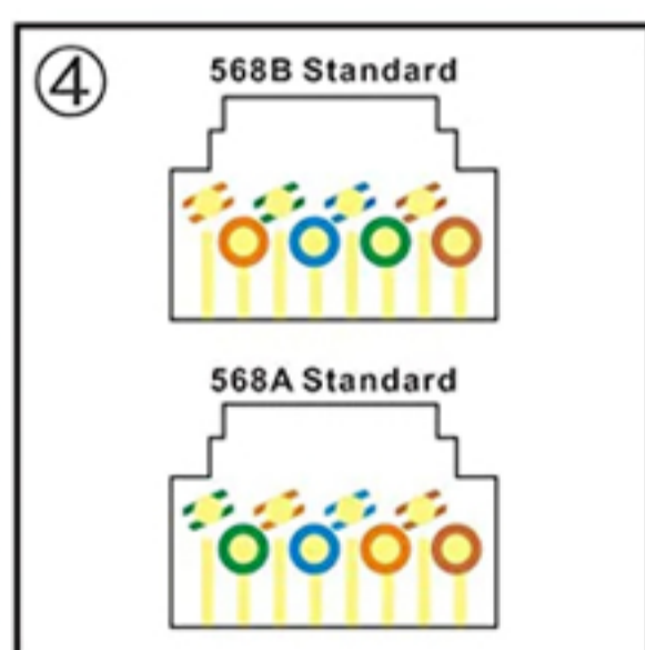
④ Place the wires in T568A or T568B order
